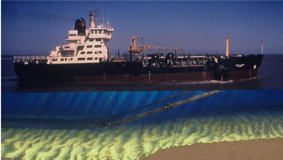
(2) connect to a pump-out facility (**picture**) where the material can be pumped via pipeline to a placement area.
